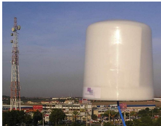
Fig.3 Multi-beam switched antenna (3.5GHz) from MPA ltd.
